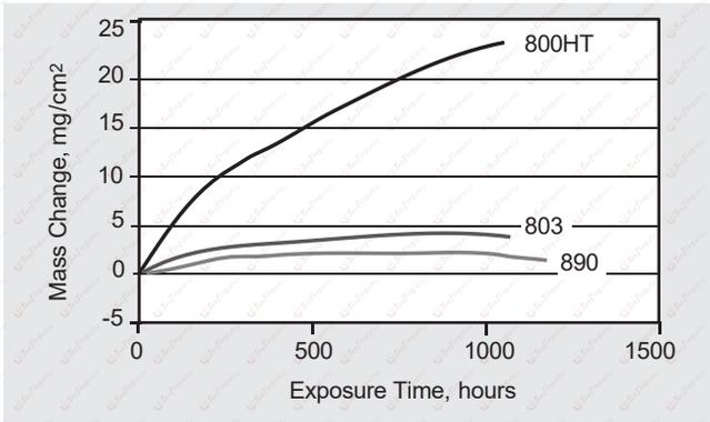
Figure 4. Mass change results after exposure in an oxidizing-carburizing atmosphere comprised of H<sub>2</sub> - 5.5% CH<sub>4</sub> - 4.5% CO<sub>2</sub> at 1000°C.
