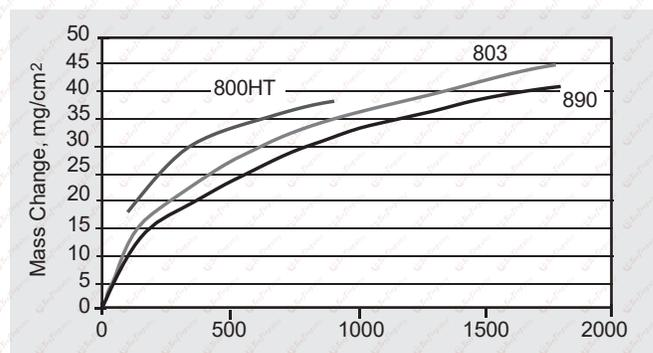
Figure 3. Mass change results after exposure in a carburizing atmosphere comprised of H<sub>2</sub> - 1% CH<sub>4</sub> at 1000°C.
