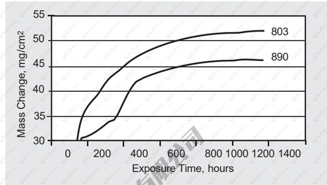
Figure 5. Mass change results after exposure in a carburizing atmosphere comprised of H<sub>2</sub> - 1% CH<sub>4</sub> at 1100°C.
